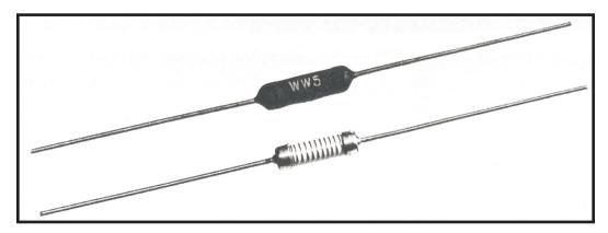
Tolerances of the WW series range through all the standard groupings from 5% down to .01%. Our standard temperature coefficients are  $\pm 90$ PPM on values from zero to 1 ohm,  $\pm 50$ PPM on values from 1 ohm to 10 ohms and  $\pm 20$ PPM on values above 10 ohms. Other special TCs are also available at the customer's request. An example:  $\pm 6000$ PPM,  $\pm 50$ PPM.
